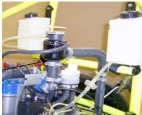
Older style (prior to 2009), Coolant and Oil Reservoirs. Caps have small nipple on top for safety wire
