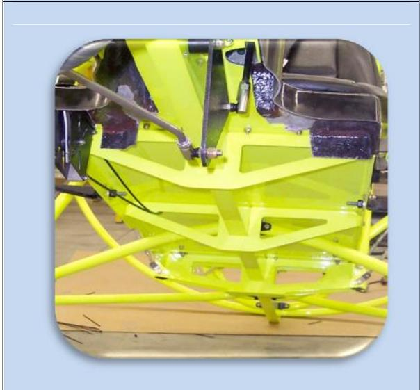
than previous models that use heavier and more tubes and brackets. The fewer tubes and brackets all feed back to the objective of being as light as possible, while not compromising strength. We have also avoided the use of heavier seats, molded body work and many other items that some manufacturers market to appeal to some potential buyers who might not be well informed about the downside of heavier options.
