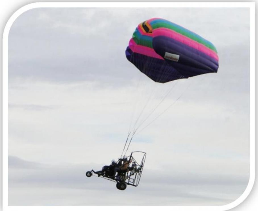
While many owners of our experimental light sport certified aircraft are flying with the elliptical canopies, we have steadfastly refused to achieve a slightly higher level of performance in exchange for what we consider the safer and easier to fly rectangular canopies. And therefore we do not offer the elliptical wing.
